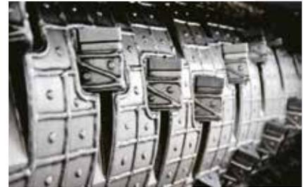
The ZTS and ZTTS shredders are equipped with a large diameter flat rotors with weld on hard facing. The knives are fixed in special knife holders fitted in machined pockets.
